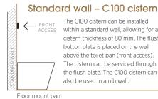
The C100 cistern can be installed within a standard wall, allowing for a cistern thickness of 80 mm. The flush button plate is placed on the wall above the toilet pan (front access). The cistern can be serviced through the flush plate. The C100 cistern can also be used in a nib wall.
